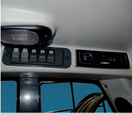
Easy access button panel for headlights, windshield wipers and bluetooth® radio.
