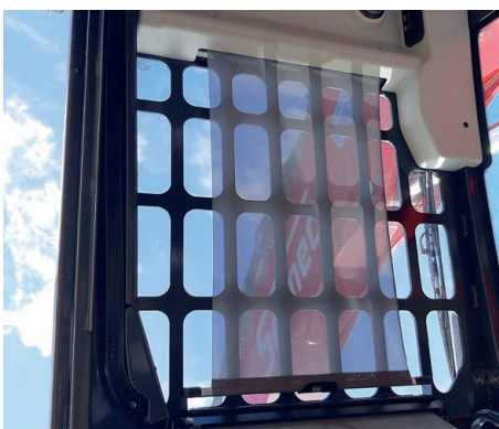
Roll-up sun blind and wiper on the roof
