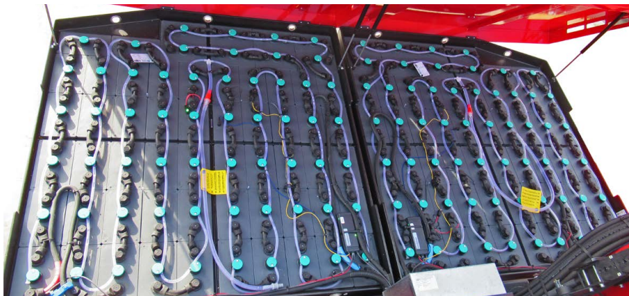
Each of the 2 high-efficiency batteries is composed by 60 elements for a supply of 120 V at 930 Ah, for about 8 working hours.
