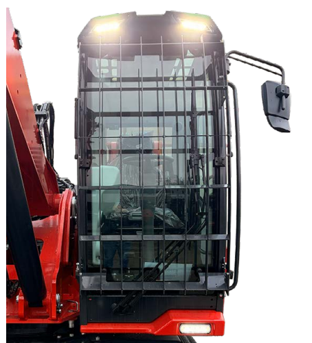
3 Standard LED headlights on cab.
