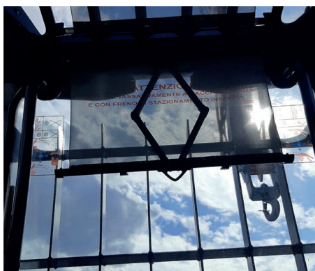
Front-mounted roller sun blind.
